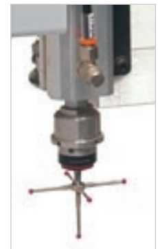
The cross-head thickness tracer enables operators to measure panel dimensions with absolute precision.
